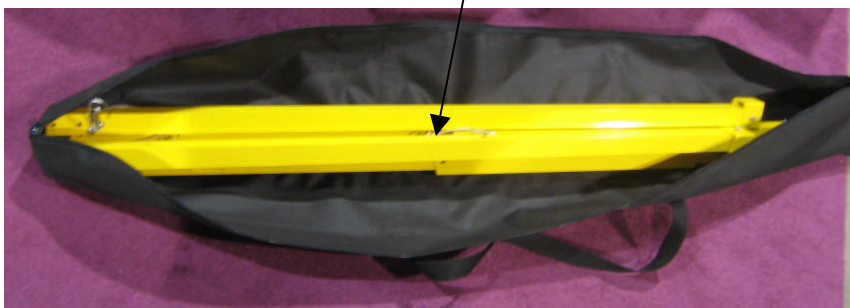
Vertical leg structure including cross-stabilizers
