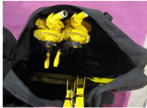
Pumps and "T" base parts. Velcro® strips inside wrap around to hold pumps and base "T"s in place
