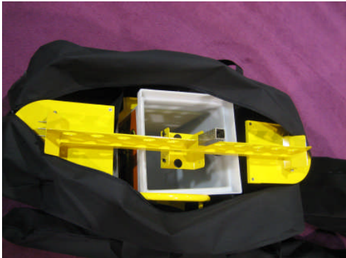
Water tank and tray, bucket structure (plus, hoses stored in water tank)
